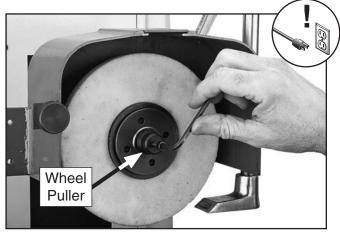
Figure 37. Using wheel puller.
